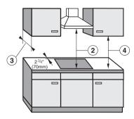
There must be a safety distance of at least 30" (760 mm), ② between the appliance and any objects above it. The overhead cabinet depth, ③, if unprotected, must not exceed 13" (330 mm). The minimum distance of combustible surfaces located above and to the sides of the cooktop, ④, is 18" (457 mm).
